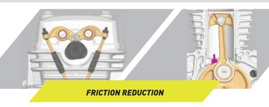
The piston cooling jet reduces friction and maintains optimum engine temperature. The offset cylinder, rocker roller arm fitted with needle bearing further reduces the frictional losses in the engine.
